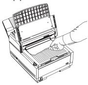
3. Push the buttons on the side of the copy stacker until you hear a click. Lift the copy stacker out of the way.
